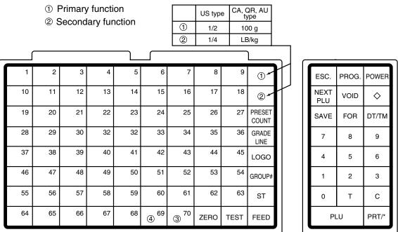
**NOTE:** 1. The numbers 1~70 indicate the speed key layout, but the actual keys have no number. Pressing the 💿 key enables another 70 PLUs assignment.
